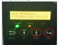
If the battery voltage and SOC are not displayed, the communication fails.
